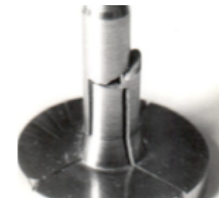
Picture 2 – Destruction of a moving upper piston at a temperature of 100 K and a pressure of 3000 MPa
